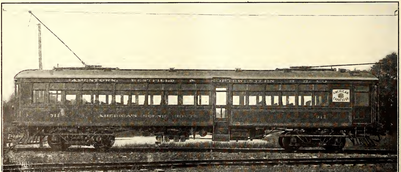
JAMESTOWN CARS—THREE-COMPARTMENT INTERURBAN CAR WITH OFFSET CENTRAL VESTIBULE
